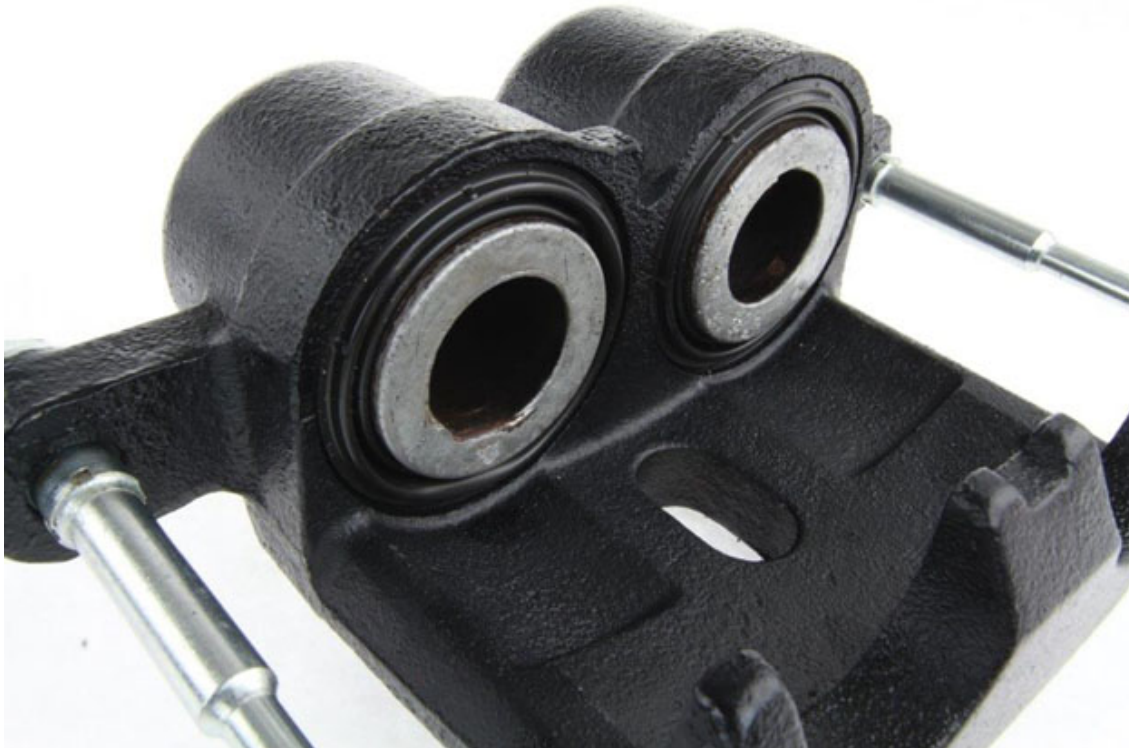
Image 1: Damaged phenolic pistons have been reused in this caliper.
