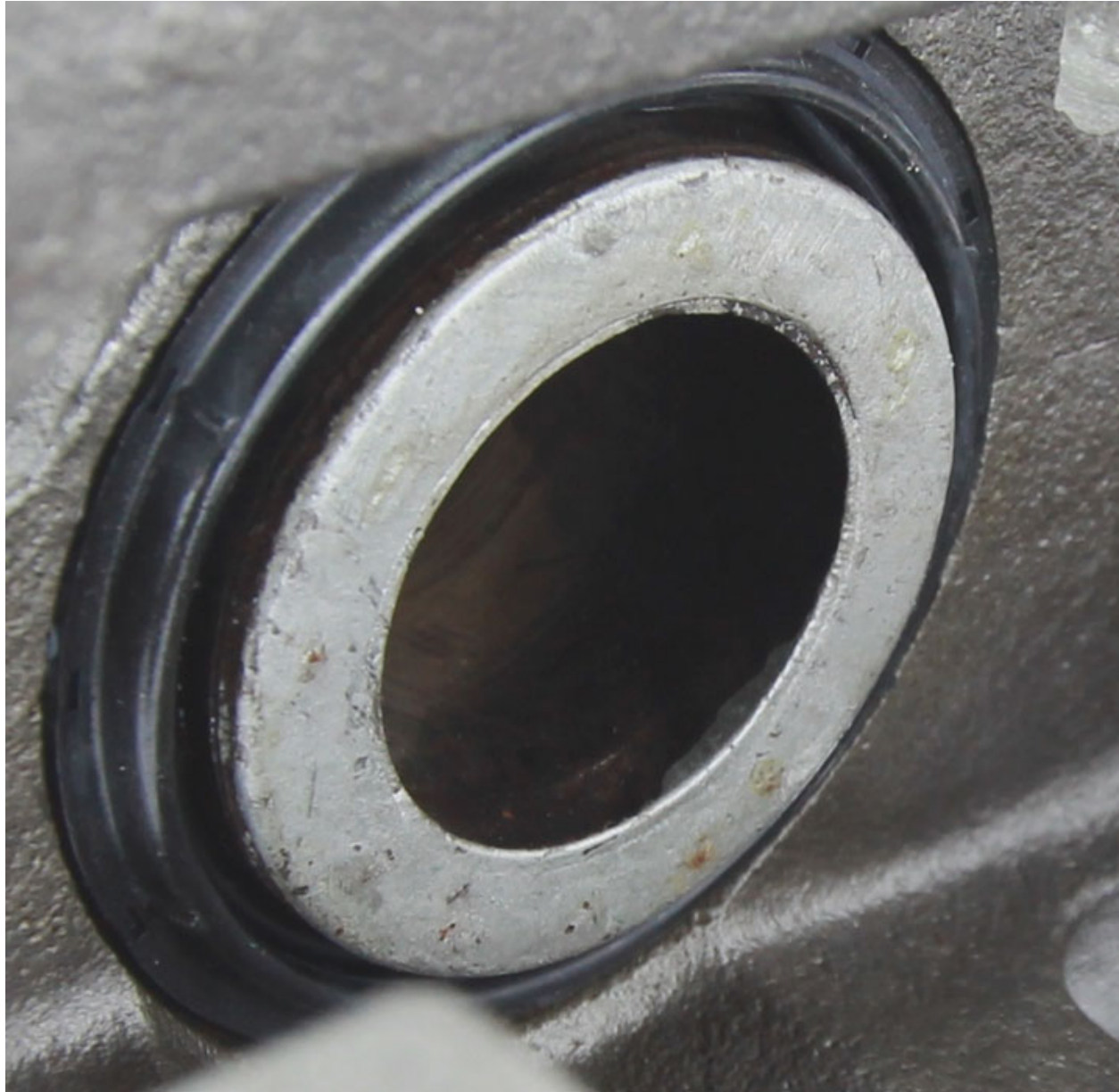
Image 6: Pitted and corroded caps
