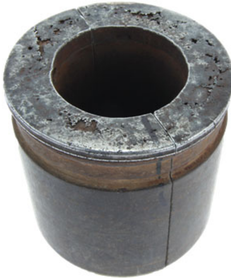
Image 4: Damage to this used piston from an external visual inspection appears to be minimal and contained to the steel cap.
