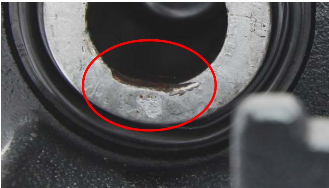
Image 3: Dented and pitted caps; most likely the result of forcing the piston into the caliper with pliers
