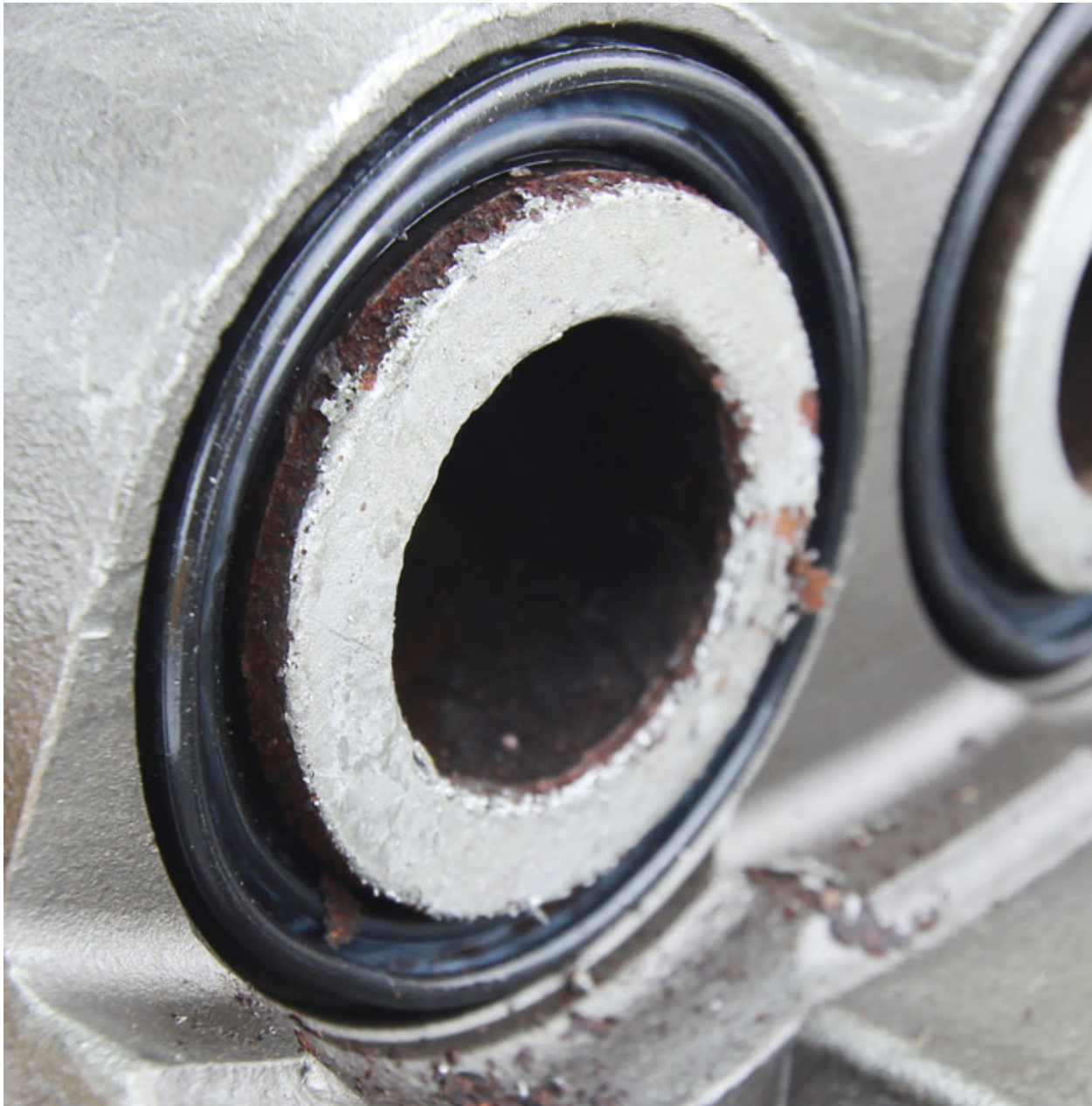
Image 8: Severely corroded cap is flaking apart
