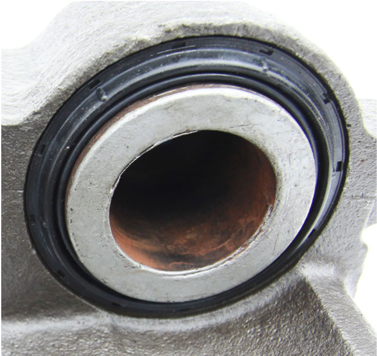
Image 7: Severe corrosion of the cap depositing rust into the piston
